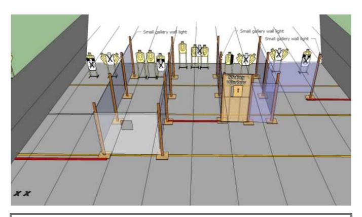
**SETUP NOTES:** Low intensity lighting will positioned as shown. Walls run completely to the floor. Mark target stand locations with chalk.
